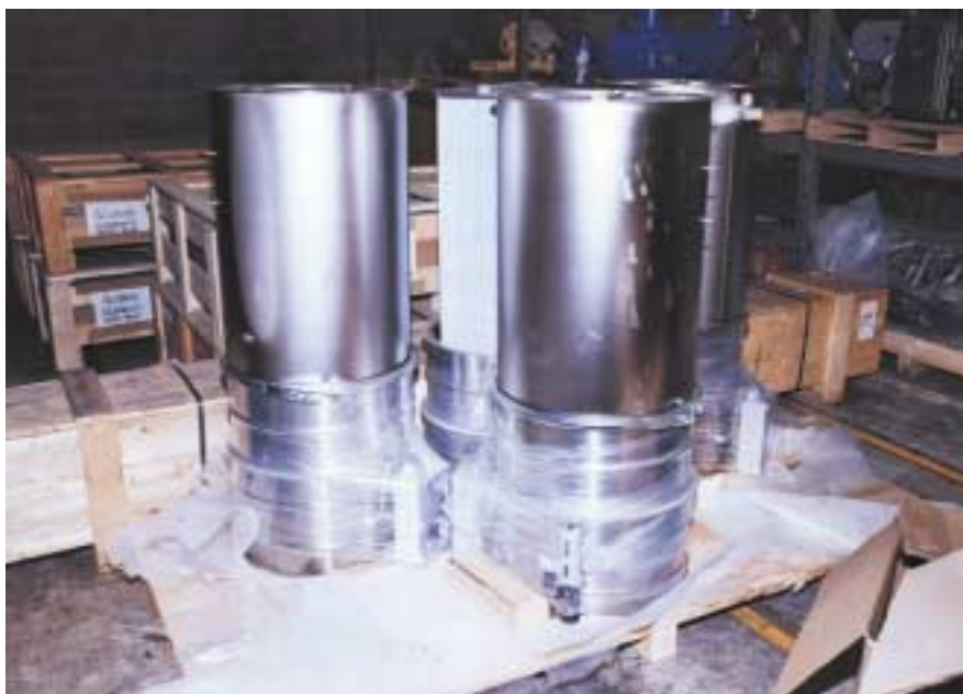
Six to eight sintered-plastic filter elements were installed on each dust collector.
