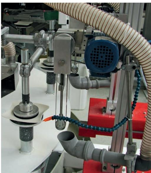
**Fig. 3** Dust capturing hoods at a fettling/rim treatment machine for isostatically pressed articles
